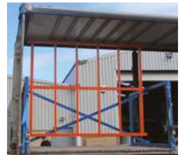
The frame has a hinged top rack and can form a second deck (above) or be lowered into the vertical position (right)
