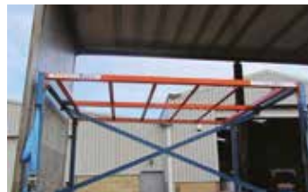
The frame has a hinged top rack and can form a second deck (above) or be lowered into the vertical position (right)
